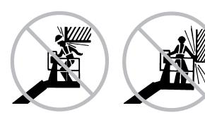
Be aware of crushing hazards when grasping the platform guard rail.
